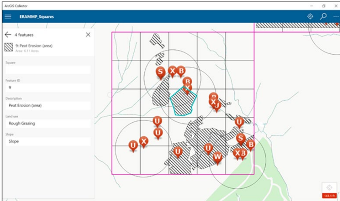
Figure 1-2 An example of the style of map that the field surveyors used to record SED features and validate the presence of EO-mapped features. Features were recorded within a 200 m radius of each X-plot in the survey square. Shapes with dashed shading indicate EO-mapped features, which when clicked, provide information of the expected SED feature (in this example, peat erosion). Taken from ERAMMP Report-70 (Tye, et al., 2023).
