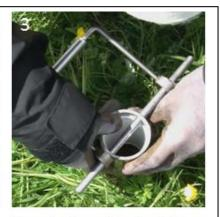
Place plastic core in coring device
