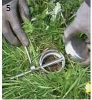
Knock coring device in until cross bar is flat on surface
