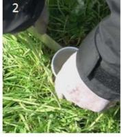
Use knife to cut roots around core
