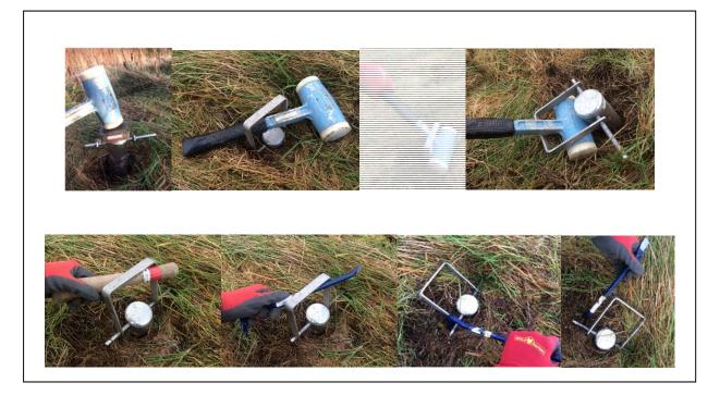
Figure 1.3.3.2 – Tips & tricks for pulling out the corer from hard/dry soil
