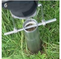
Remove from soil, extract core, cap, red at top, black at bottom, bag
