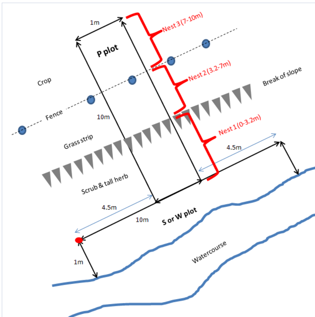
Layout of P plot. The red blob shows the location of the differential GPS point for the S or W plot. The nest lengths here are an example only. In reality the number of nests and their sizes will vary at the surveyor’s discretion up to a total of 6 nests i.e. from 0 to 5 as for the X plots.
